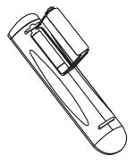
Replace battery cover by aligning and inserting the two tabs into the holes. Press battery cover into place until it "clicks" closed.
