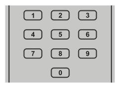
Using the direct-entry numeric keypad (0 to 9) causes the C 546BEE to jump directly to the beginning of a numbered track and commence play. Thus, to play Track 5, simply press "5". To play Track 20, press "2" and "0".
