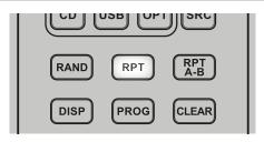
A particular track or file can be repeatedly played back by pressing [RPT] button. Toggle this button to repeat a track/file, folder, all tracks or all files. Corresponding icons like REPEAT, REPEAT FOLDER, or REPEAT ALL will be illuminated in the VFD as the particular repeat mode is selected. Turn off repeat mode by pressing the REPEAT button until the REPEAT icon is extinguished in the VFD.
