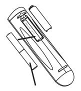
Press batteries into opening. Ensure correct fitting is observed.
